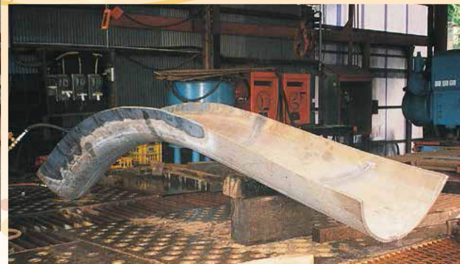
Bottom oil drilling equipment Jack-up rig for the chord Thickness (76.2mm)distortion up
