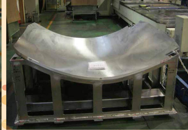
Metallurgy tool song processing of aviation parts production (aluminum plate thickness 35mm)
