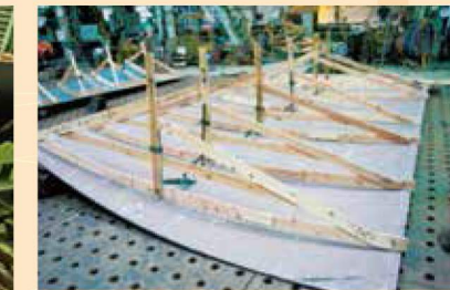
Metallurgy tool song processing of aviation parts production (aluminum plate thickness 35mm)
