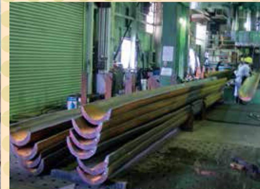
Bottom oil drilling equipment Jack-up rig for the chord Thickness (76.2mm)distortion up
